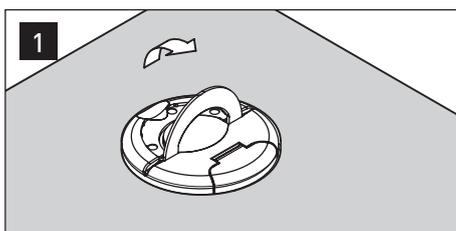
To use the Pop-up Socket, gently lift up the silver handle on the top cover until all socket outlets are exposed and the green stop/release button clicks and locks the unit in place.
