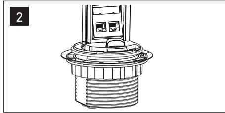
The locking ring with rubber washer is supplied in the packaging. If attached to the mounting collar, remove it by rotating it in an anti-clockwise direction prior to lowering the unit into its final location.
