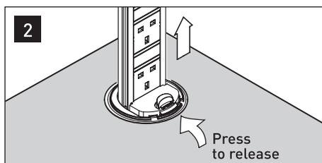
Press the master switch on. A green light confirms that power is available. You can use all power sockets. The unit can be retracted in position by pressing the green stop/release button and push the unit down until it's flush with the surface. And leaving the engaged cables on the window of the top cover.
