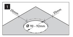
Cut out 90 - 92mm diameter hole in work surface. Allow minimum 25mm clearance around the cut hole. When choosing location, select a surface between 10mm and 50mm thick.
