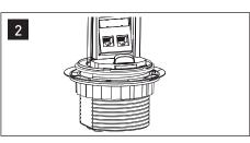
The locking ring with rubber washer is supplied in the packaging. If attached to the mounting collar, remove it by rotating it in an anti-clockwise direction prior to lowering the unit into its final location.
