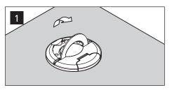
To use the Pop-up Socket, gently lift up the silver handle on the top cover until all socket outlets are exposed and the green stop/release button clicks and locks the unit in place.
