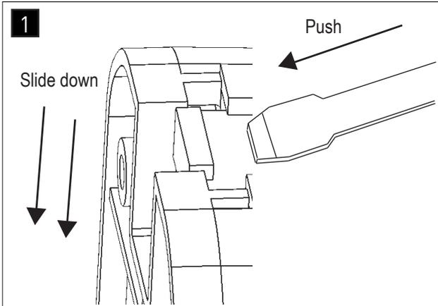
Use a flat edge screwdriver to release the mounting plate from the back of the block at the bottom of the fitting. Push the screwdriver edge against the lock (see diagram above) and slide down to release the mounting plate.
