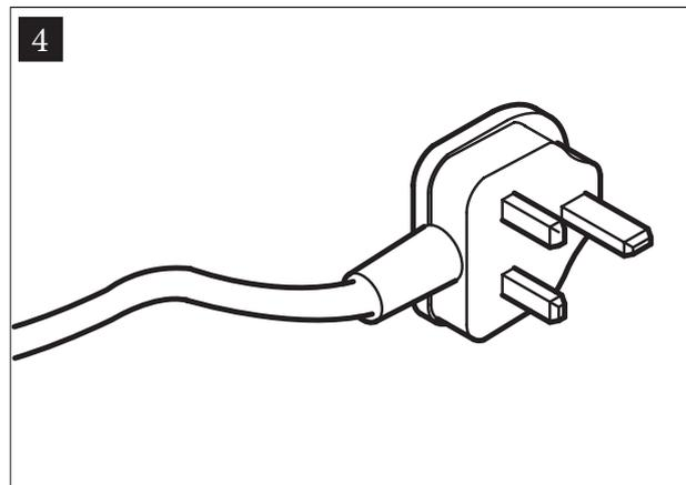
Finally wire the 1.5m cable supplied to the 240V mains supply or 13A plug top.
