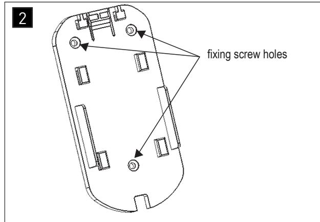
Mark the position for the mounting plate on the back of the headboard. Once marked up, secure using the provided fixing screws.
