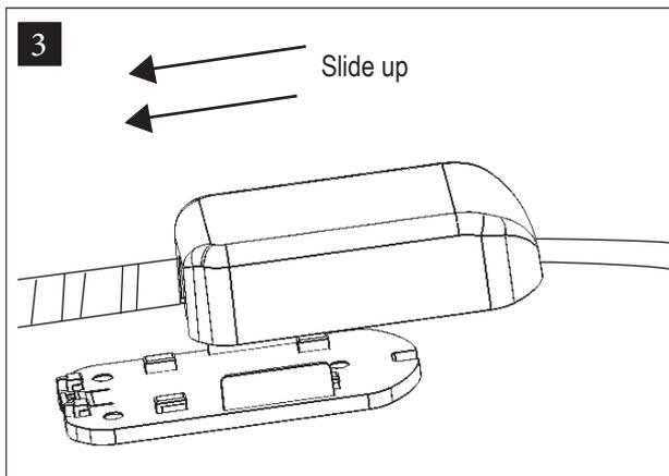
Re-attach the housing to the mounting plate by pushing the housing onto the plate and sliding upwards until the lock is secured.
