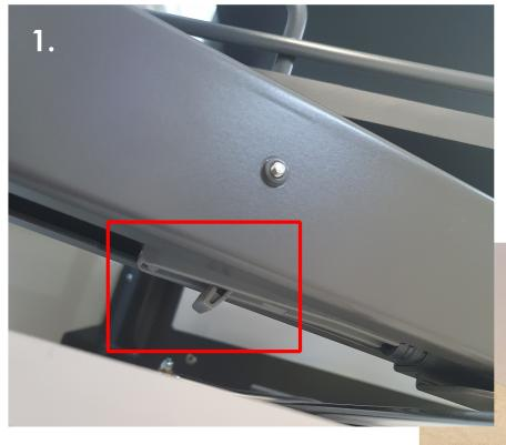
Make sure the soft closer is set forward in this position (if not working correctly this will be set further back)
