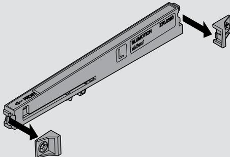
2 Rotate end brackets 180° and re-attach
