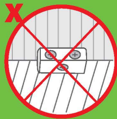
Incorrect fixed bracket
