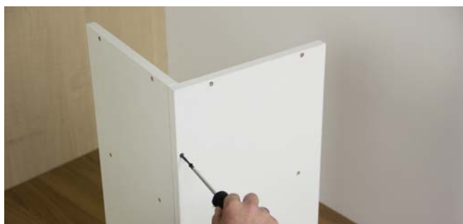
Screw larger panel into smaller panel using 1 3 / 4 black screws (Included) Pre-Drilled
