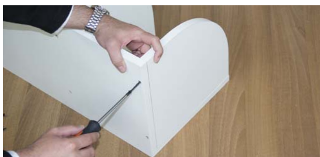
Screw the 4 shelves on the other side using 1 3 / 4 black screws (Included) Pre-Drilled
