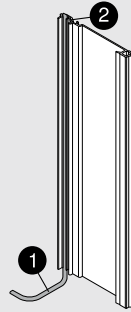
Bracket profile with both cables
