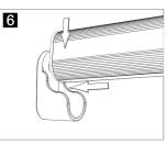
Slot light unit into bracket cradle.
