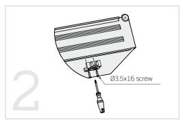
Support the fixing bracket and screw it on with the  $\emptyset 3.5 \text{x} 16$  screws.
