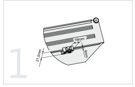
Mark the centres of the indicated measurements. It is recommended to mark and drill side holes with a  $\emptyset1.5$  bit.
