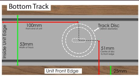
One disc should be placed 100mm from each side of the unit with the remaining discs spaced equally over the unit's width (Fig. 1)
