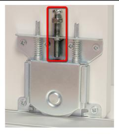
Taking the weight of the door in the track, use the middle bolt to adjust the door height.
