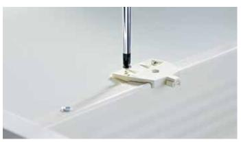
Two screws in the bottom and one in the drawer profile are required. All three are required for proper function
