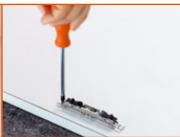
Attachment of symmetrical front fixing brackets to the front.
