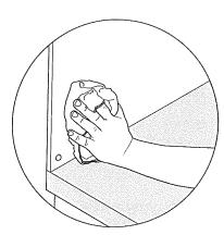
Once the sealant has cured clean the splashback with a soft damp cloth.
