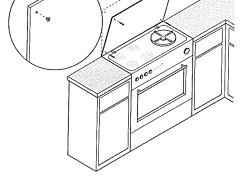
Drill holes approximately 35 mm deep into the wall using a 6 mm drill bit.
