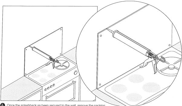
6 Once the splashback as been secured to the wall, remove the packing shims.
