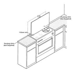
Firstly offer up the back of the splash back to the worktop/wall placing it onto the two 3 mm packing shims (not supplied) to check the fit. Then mark the 4 fixing holes with a pencil.
