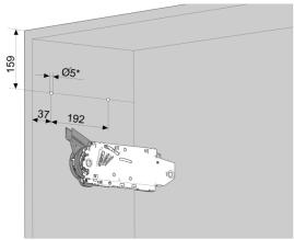
\* Drilling depth 5 mm
