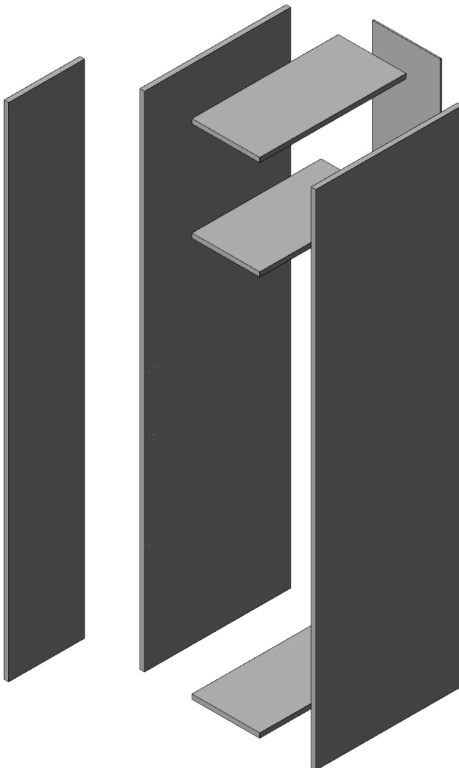
Note: 20mm drilling point for horizontal plates, 37mm for cruciform (we recommend to use 3 fixing points in either case)
