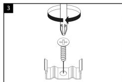
Fix the brackets to the desired position using the screws included.
