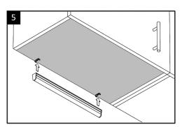
Clip the Connex into the two fixing brackets to secure it in position.
