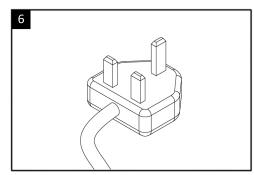
Finally, connect the Connex directly to 240V mains supply or 13A plug. If you are creating a run of Connex lights, you only need to connect the Connex at the start of the run.
