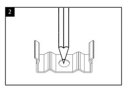
Using a pencil, mark where the fixing brackets will be positioned - one at either end to take the weight of the light evenly.
