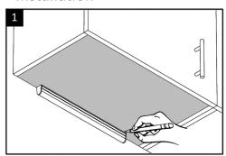
Using a pencil, mark the desired position for the Connex under the cabinet.
