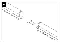
If you are installing a run of Connex lights, remove the end-caps and connect the lights by inserting the male-end into the female-end.
