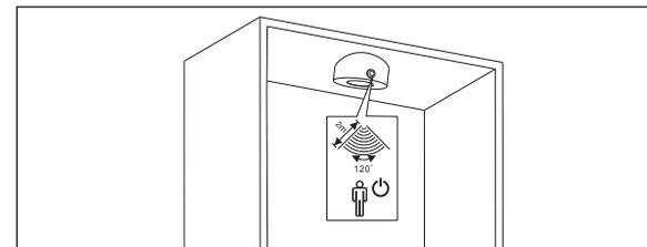
The Solus Rechargeable Wardrobe Light has a built-in PIR sensor. When the wardrobe door is opened this switch will detect motion from a distance of 2m and the light will switch on. Recharge the unit using the SE2007000 pluggable USB charger.
