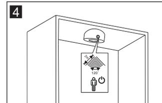
Sensor detection range & detection angle when installed.
