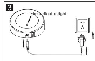
Connect the USB cable to the charger and light. When charging, the indicator light, will be red; when finished charging, it will be green. Charging time: 6 hours, continuous working time: 9.5 hours.
