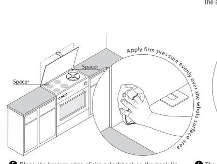
Place the bottom edge of the splashback to the back lip of the worktop / wall on the spacers provided then push the splashback to the wall and apply firm pressure evenly over the whole surface area. Ensure that the 3mm spacers are left while the sealant bonds to the wall. Finally after 2-3 hours remove the spacers.
