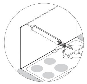
**6** The 4 exposed edges of the Splashback must be sealed with a bead of silicone sealant no less than 2-3 mm in thickness.
