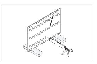
Take the Splashback away from the wall making sure to keep all corners safe from hard surfaces. Apply a generous amount of silicone to the back of the splashback, making sure not to go too near the edges. Remove the covering from the self adhesive backing.
