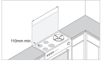
• Firstly check the dimensions. The minimum distance from the back of the rear hobs to the wall should be no less than 110 mm.
