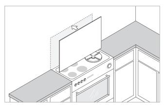
Firstly offer up the back of the Splashback to the worktop /wall to check the fit. Use the spacers provided to achieve a good fit. There needs to be a gap of 2-3 mm around all 4 sides.
