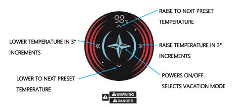
If the electronic instant hot water appliance is empty of water and is turned ON then this will be automatically sensed, the heating element will not energise and the "lack of water" indictor will be flashing on the display panel shown by the flashing of the E3 warning. code.
