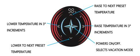
Pressing the temperature buttons above will set the temperature. <> will be move by  $1^{\circ}$  C and  $^{\wedge\vee}$  will move up and down the presets from 98Cmax. 97; 96 95; 90; 85 and 75C. When heating the red segments will pulse on and off . After processing validation checks the tank it will start to heat up after a delay of 10 seconds.
